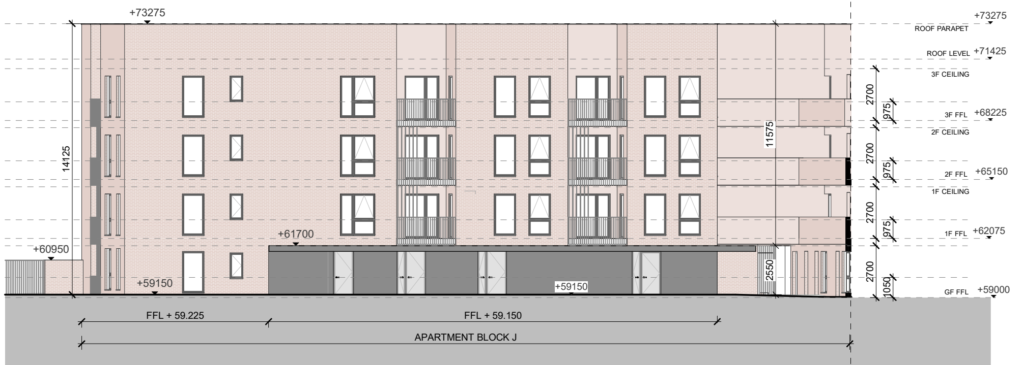
PROPOSED ELEVATION 05 - APT BLOCK - CLUSTER J - EAST 1:200
